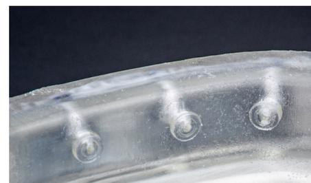
Photo 3: Device adopts micro-scale mist to remove plaque
