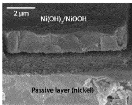
Fig. 1 Example 1:  $Ni(OH)_2/NiOOH$  deposited on a passive layer (e.g. Ni) by anodic electrodeposition
