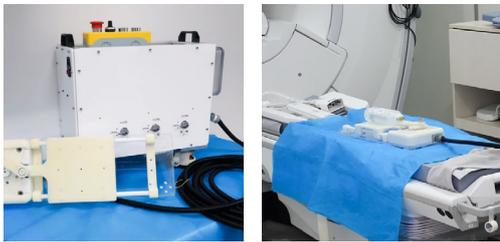
(Left: MR-safe motion platform with controlling console; Right: motion platform inside MRI room)
